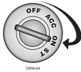
Turn the ignition key on and press the Valet switch the preset number of times within 15 seconds. If the system does not disarm, you may have waited too long to press the Valet switch; turn the ignition off and repeat the process.
