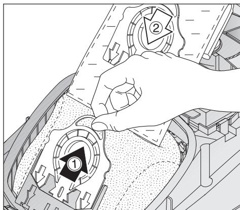
The lid will not close without a dustbag in place, or if the dustbag is incorrectly fitted. Do not force it.
