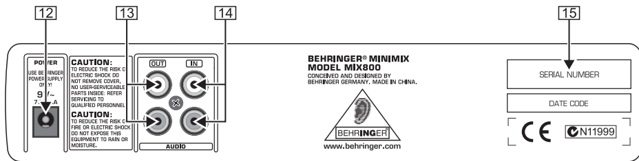
Fig. 2.2: Rear panel connectors of the MIX800
