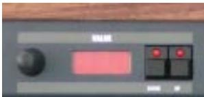
With the Data-Wheel (on the left) or the DOWN/UP buttons you can set the parameters of the Configuration Strip, like i.e. MIDI-Channel or Volume. Choose between the monophonic / polyphonic mode by pressing DOWN and UP button at the same time (MONO/POLY). The display will show "of" for monophonic and "on" for polyphonic mode.
