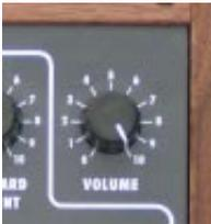
Here you can adjust the master volume for the Synthesizer. As this wheel also regulates the volume of the instrument before effects passing, you can also use it to meter the implemented effects, i.e. to avoid distortion when using the Flanger with a lot of feedback.
