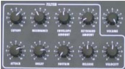
To modulate the Filter you can use an assignable envelope curve, the keyboard envelope curve and the sources of the modulation matrix.
