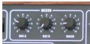
The third volume control regulates the volume of the noise signal (in this case white noise).
