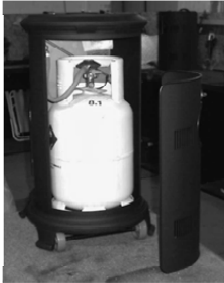
Rear view of stove showing the gas cylinder, the rear door and the top cover
