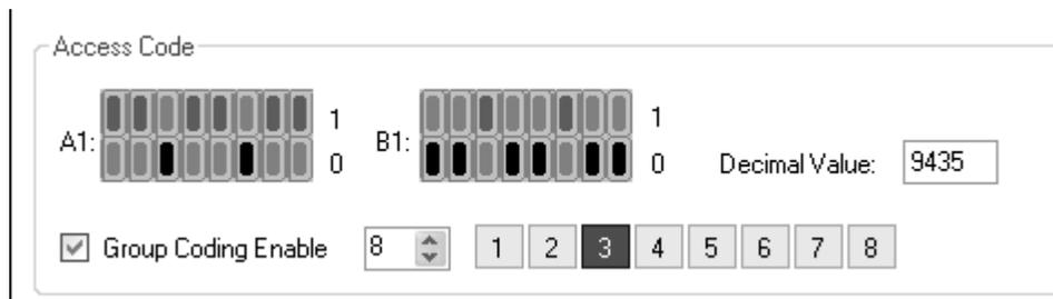
Enter each access code that the receiver should accept by clicking each number button and setting that access code as above.
