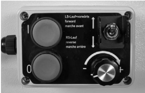
The control box has a magnetic base enabling it to be positioned anywhere on the lathe
