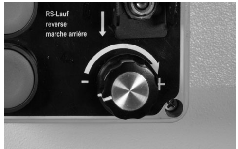
The Speed Control Knob, enables you to increase or decrease the speed of the spindle
