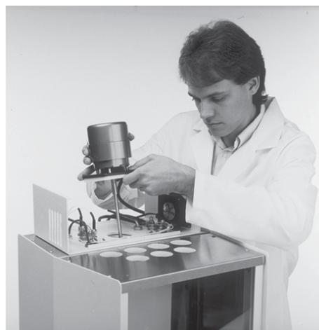
Figure 9: Installing motor-stirrer
