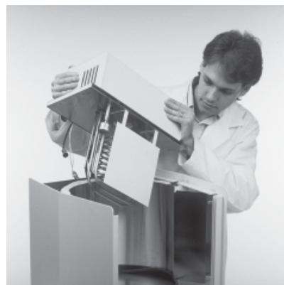
*Figure 4: Removing back top cover*
