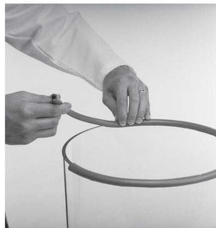
Figure 6: Seating the gasket
