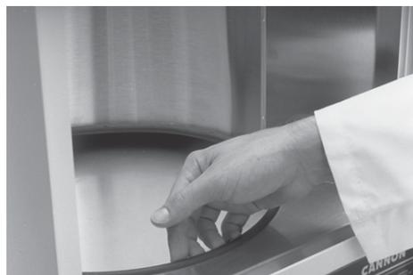
*Figure 5: Seating the support ring*
