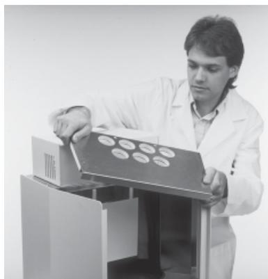
*Figure 3: Removing front top cover*
