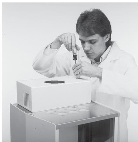
Figure 8: Removing heater housing
