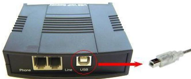
The other end of the USB cable must be connected to a USB port on your computer as shown below,
