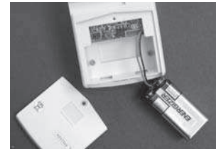
Insert 9V alkaline battery to the sensor
