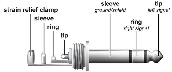
Fig. 2.5: Stereo plug for headphones connection
