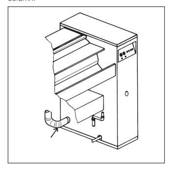
To prevent the build-up of condensation in an upward sloping exhaust ducting, a 3-5 mm ø condensate drain should be fitted at the lowest point.
