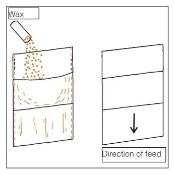
■ To apply wax with the wax cloth, place some granular wax in the pouch of the wax cloth, close the pouch and feed the cloth through the ironer at 180 °C with the non-rubberised side facing the heater plate. Use the wax sparingly to avoid the roller cover becoming too smooth.
