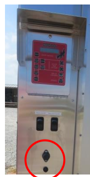
Figure 3-FEC500 & FEC750 Foot Pedal Plug-In Front Bottom of Controller
