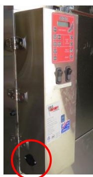
Figure 2-FEC300 Foot Pedal Plug-In Side of Controller
