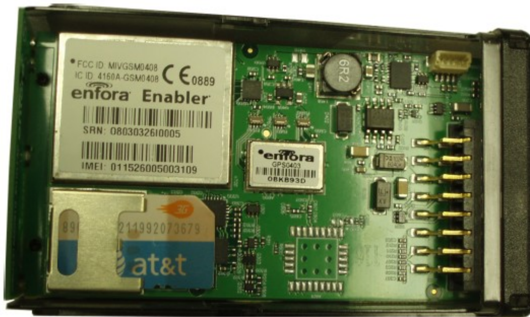
Figure 7: Internal view of the GPS-208. Note the orientation of the SIM card.
