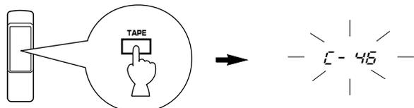
You can select any of four tape lengths by pressing the **TAPE** button.
