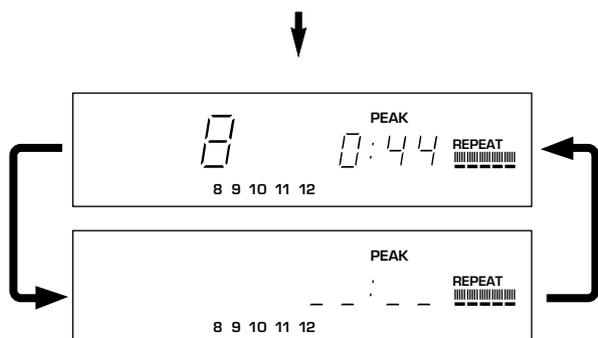
Next, the part where the source level peaks is repeatedly played. Adjust the recording level on the tape deck listening to this sound.
