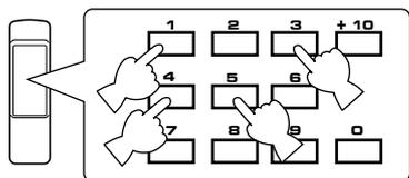
\* Programmed track numbers light up on the display. You can select a track which can be programmed for the remaining time of (the side of) the tape from track numbers flashing on the display, but you cannot select a track number extinguished from the display.
