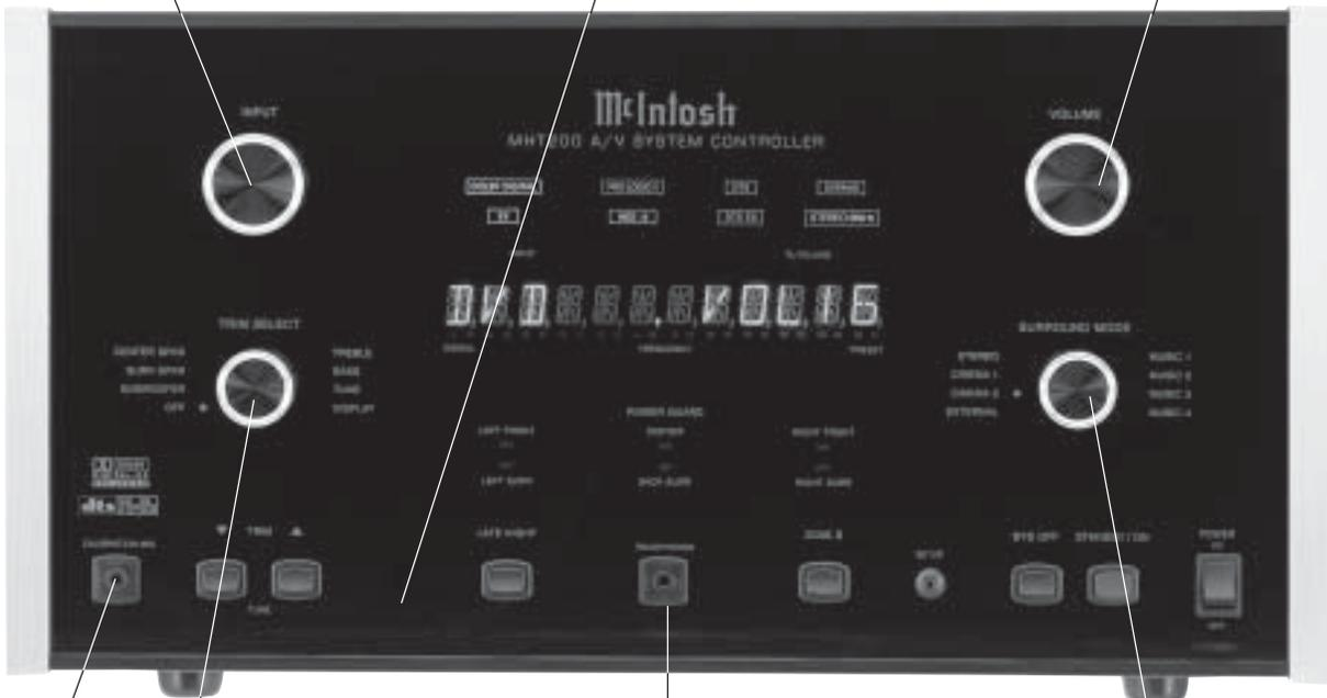
CALIBRATION MICrophone Input for adjustment of Loudspeaker Levels and Time Delay
