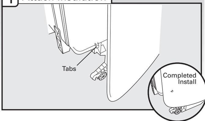
Using the precut slots in the insulation, fasten the insulation over the molded hooks on the tub. Be sure to fasten the insulation down on both sides of the tub.
