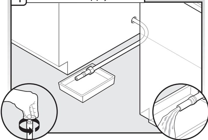
Slowly turn water shutoff valve to "ON" position. Flush water into a shallow pan until clear to get rid of particles that could clog the inlet valve. Turn shutoff valve to "OFF" position.
