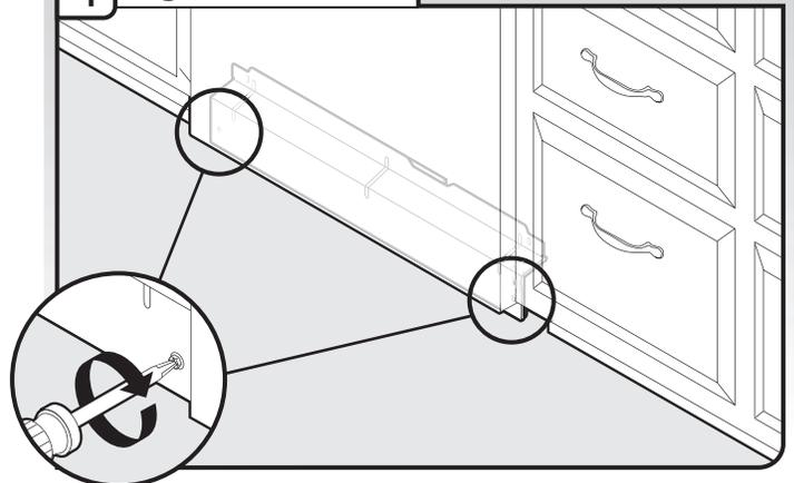
Tighten access panel screws.
