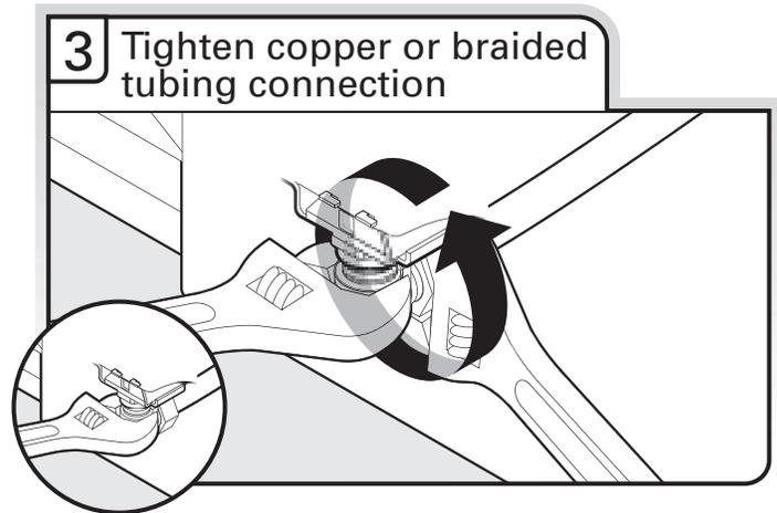
Hold the 90° elbow fitting still with one adjustable wrench and tighten the nut with second adjustable wrench.
