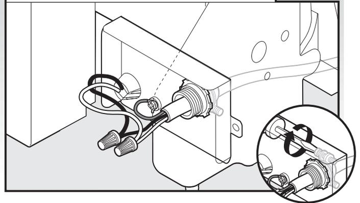
Tighten strain relief screws to secure cable.
