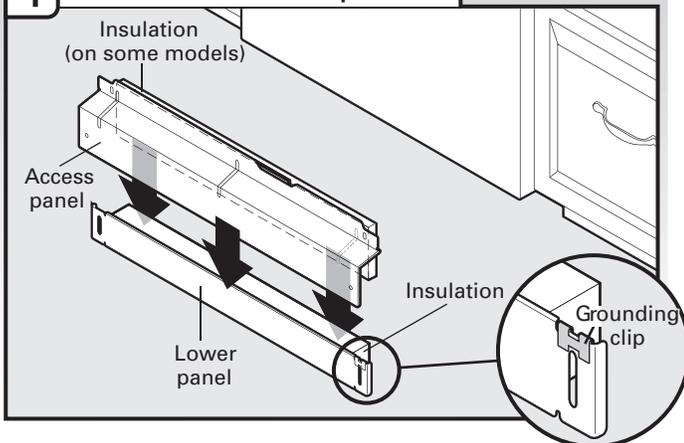
Check that grounding clip is attached to the lower panel. Position the lower panel behind the access panel. On some models there is insulation on the access panel which must fall behind the insulation on the lower panel.
