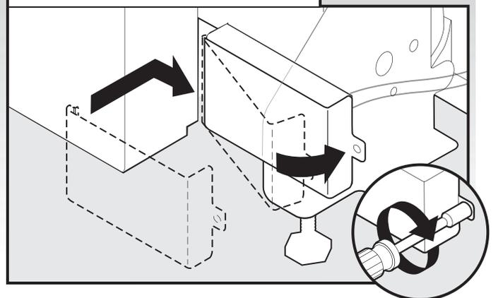
Place wires inside terminal box. Insert tabs on left side of cover. Make sure wires are tucked inside box. Close cover ensuring wires are not pinched. Use 1/4" nut driver and previously removed screw to secure cover.
