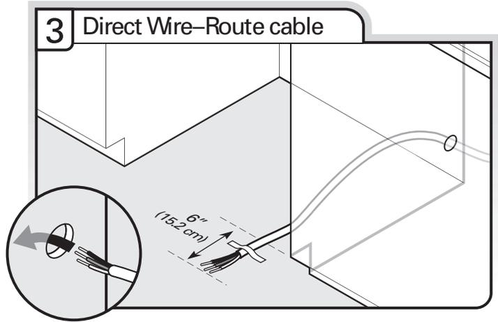
Route cable from power supply through cabinet hole (cable must extend to the right front side of cabinet opening).
