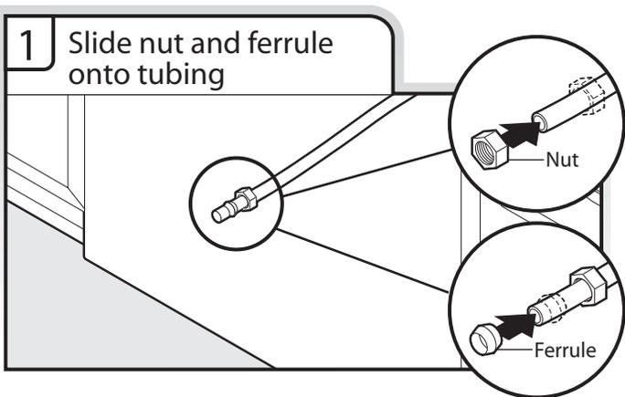
Copper tubing only: Slide nut then ferrule onto copper tubing about 1" (2.5 cm).
