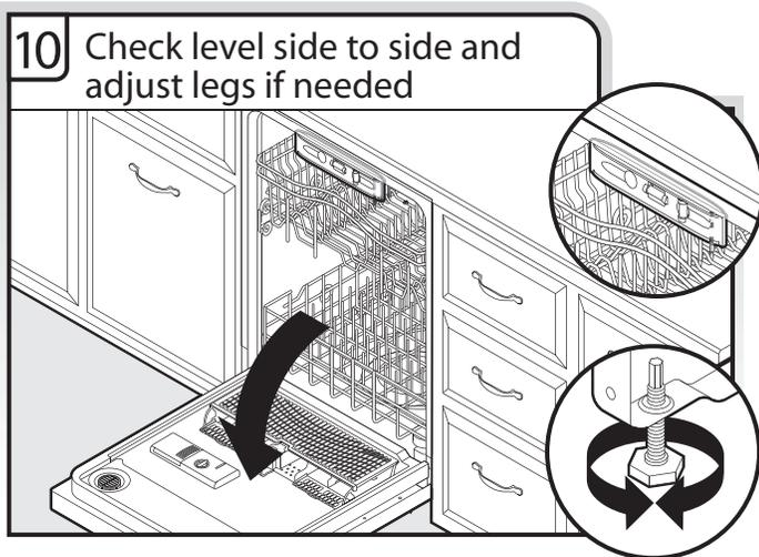
Place level against top front opening of tub. Check that dishwasher is level from side to side. If dishwasher is not level, adjust front legs up or down until dishwasher is level.
