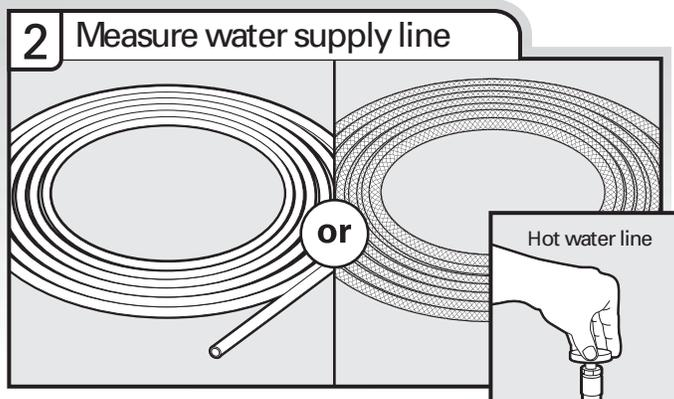
Measure overall length of copper tubing or flexible braided water supply line. Attach to the hot water line using a connection configuration that is in compliance with local codes and ordinances. The water line to the dishwasher should have a manual shutoff valve.
