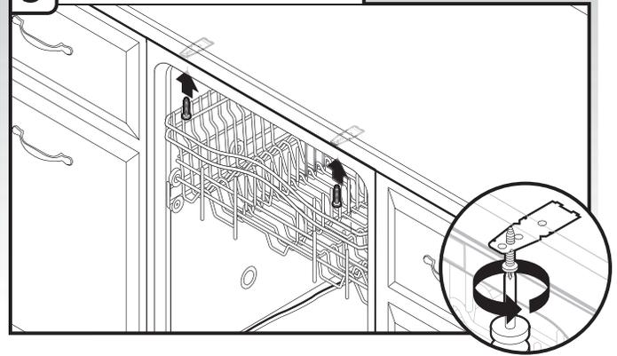
**NOTE:** Do not drop screws into bottom of dishwasher.
