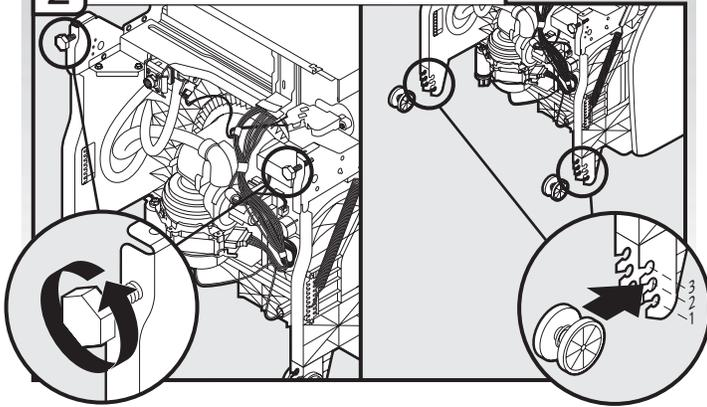
Turn both leveler legs to the same height. Put wheels in the required position determined from "Dishwasher Height Adjustment Chart". (To change wheel position, use a flat-blade screwdriver to pop out the wheel, then snap into the new position.)
