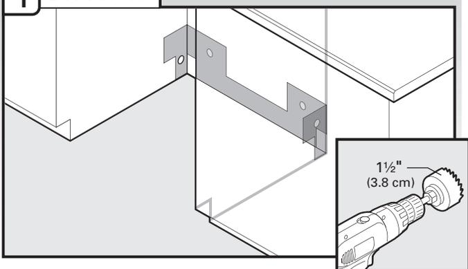
If needed, drill a 1 1/2" (3.8 cm) diameter hole in cabinet wall or side of the opening closest to the sink.
