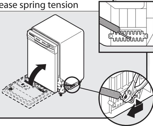
If the door closes too quickly, decrease the spring tension by moving the spring end toward the front of the dishwasher.
