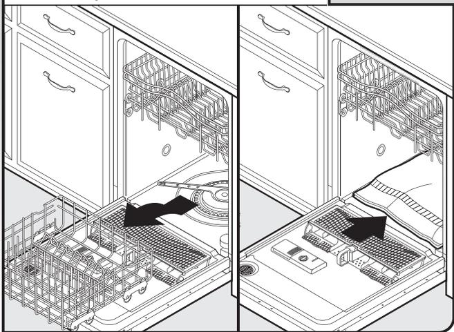
Open dishwasher door, remove lower dish rack, and place towel over pump assembly and lower spray arm of dishwasher. This will stop screws from falling into pump area when securing dishwasher to countertop.
