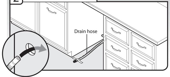
Route drain hose as shown through hole in cabinet to the front center of opening where drain connection will be made. Tape drain hose to the floor in area shown. This will keep it from moving when dishwasher is moved into cabinet opening.
