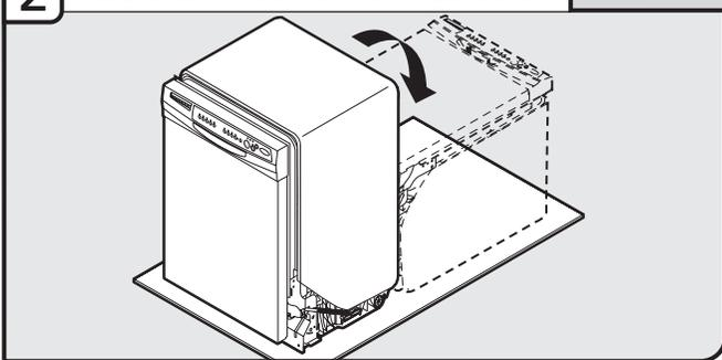
**Helpful Tip:** Place cardboard under dishwasher until installed in cabinet opening to avoid damaging floor covering. Do not use door panel as a work table without first covering with a towel to avoid scratching the door panel.
