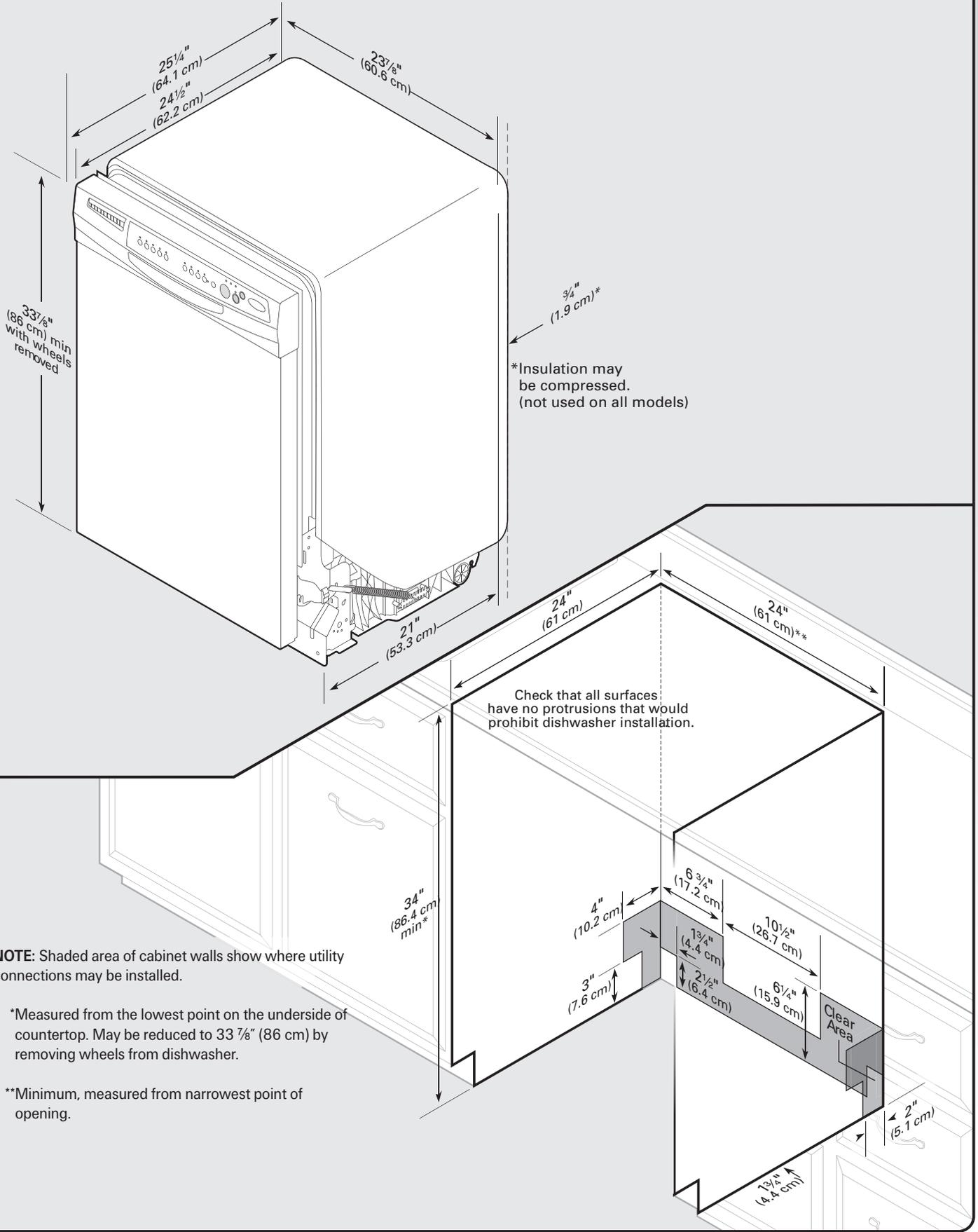
**NOTE:** Shaded area of cabinet walls show where utility connections may be installed.
