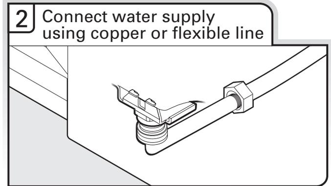
Copper tubing only: Put the tubing into the 90° elbow fitting as far as it will go (the copper tubing bends and kinks easily). Slide the nut and ferrule forward and start the nut onto the elbow threads.
