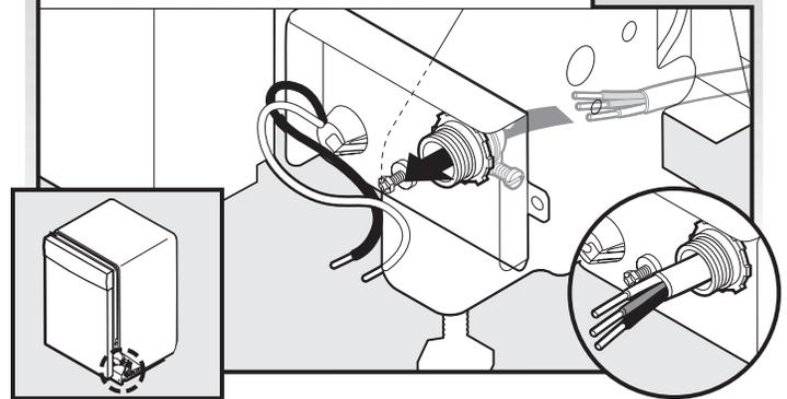
Route cable so that it does not touch dishwasher motor or lower part of dishwasher tub. Pull cable through cable clamp in terminal box.
