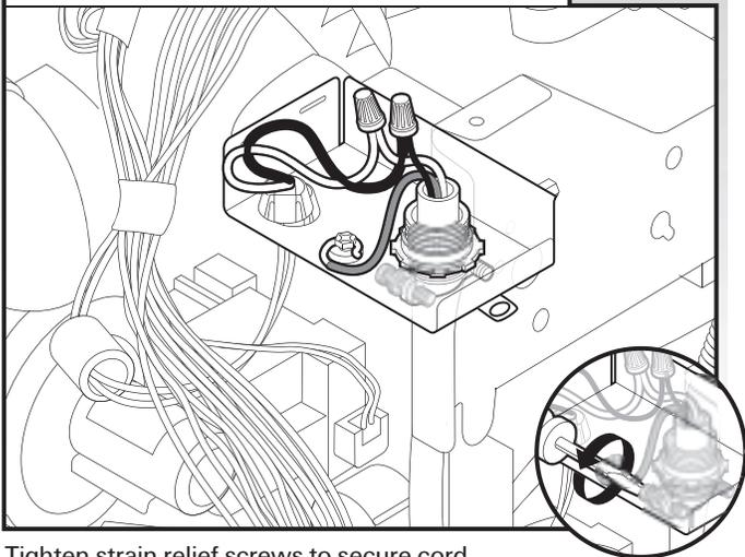
Tighten strain relief screws to secure cord.
