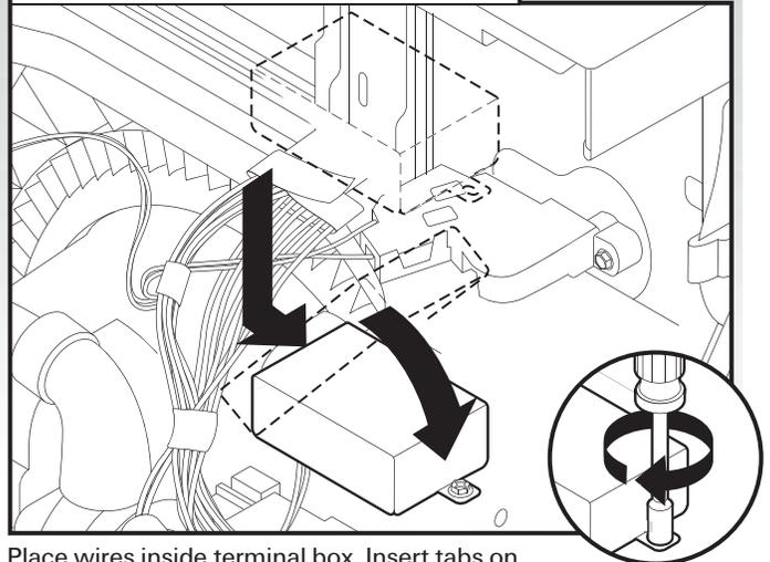
Place wires inside terminal box. Insert tabs on left side of cover. Make sure wires are tucked inside box. Close cover ensuring wires are not pinched. Use 1/4" nut driver and previously removed screw to secure cover.
