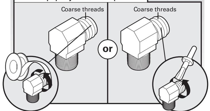
Apply Teflon® tape or pipe joint compound to 90° elbow fitting (not provided). Wrap tape around coarse threads 2 to 4 times to avoid leaks.
