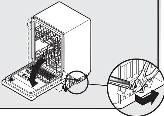
If the door falls open, increase the spring tension by moving the spring end toward the back of the dishwasher.
