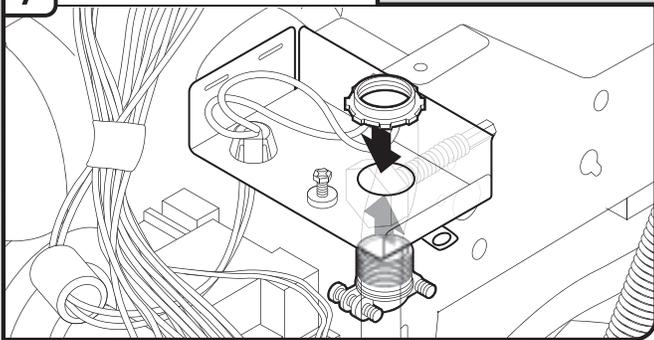
Install a UL Listed/CSA Approved strain relief. Check that the screwheads are facing to the left when tightening conduit nut. Strain relief may be provided with the power supply cord kit.
