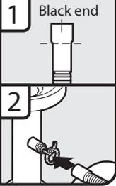
1. Connect black end of drain hose to waste tee and cut if needed.
