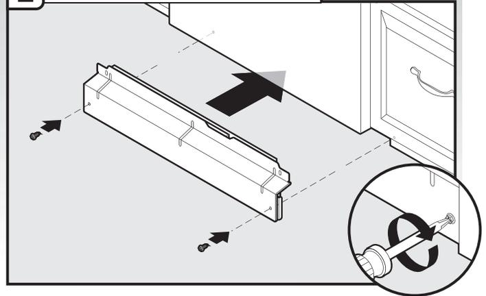
Hold the two panels together and place them against dishwasher leg. Using a Phillips or 1/4" screwdriver, reinstall the screws through the holes in the access panel and the slots in the lower panel.
