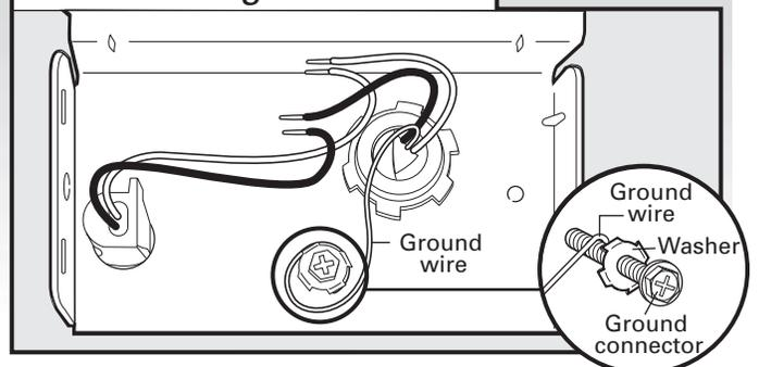
Remove the green grounding screw and place through the ring terminal of the green ground wire. Reattach and tighten the green screw.
