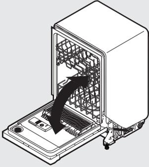
With another person holding the dishwasher to keep it from tipping, open and close the door a few times. If the door closes or falls open under its own weight, the door tension will need to be adjusted.
