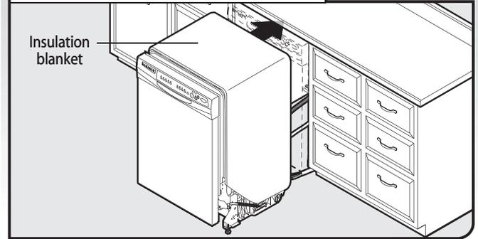
**IMPORTANT:** If wheels were removed, cover the floor when moving the dishwasher. Slowly move dishwasher completely into cabinet opening. Do not kink or pinch water line, drain hose, power supply cord or direct wire between dishwasher and cabinet. Remove cardboard from under dishwasher.
