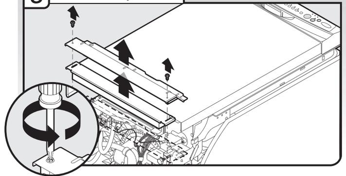
Using a 1/4" hex head socket, nut driver or Phillips screwdriver, remove 2 screws attaching access panel and lower panel to dishwasher.
