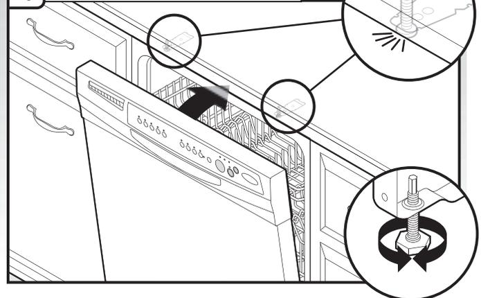
Check that top of door does not contact screws, brackets, or countertop. If it does, adjust leveling legs.
