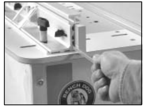
In this photo, the user is sliding the second bar into position. Be sure to tighten the subfence knobs when done!
