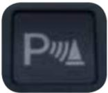
The parking sensor system uses ultrasonic sensors to detect obstructions behind the vehicle with transmission in Reverse and speed below 6 mph (10 km/h). The system notifies the driver of the approximate distance from the vehicle to the obstruction using a beep sound.
