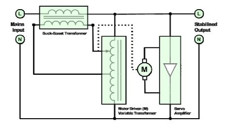
Being able to accommodate an input voltage swing of in excess of 40%, whilst still delivering accuracy on the output of 1% or better, the Servo Electronic design principle comprises a transformer having its secondary winding connected between the mains supply and the load. The primary voltage is automatically controlled through a servo motor driven variable transformer, thereby ensuring a continuous, smooth and very stable output voltage.
