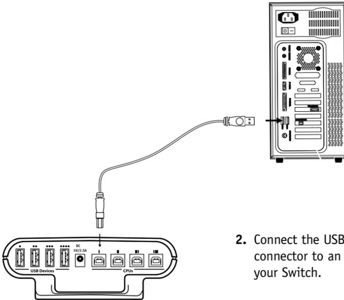
2. Connect the USB cable's B-type connector to an available port on your Switch.
