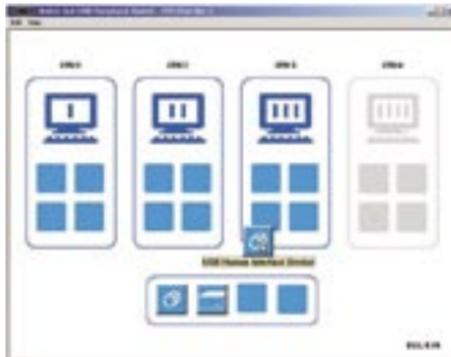
To switch USB devices from computers, drag the USB icon of the desired device to the Active Computer Port you wish to switch it to. When dragged, the software will indicate the name of the device.
