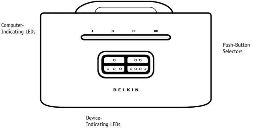
*Back View of the 4x4 USB Peripheral Switch*
