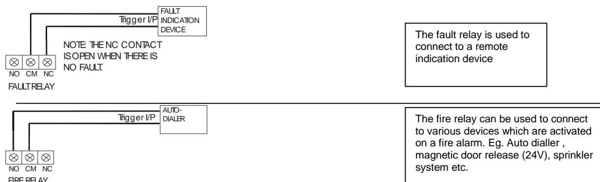
Typical auxiliary output wiring
