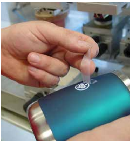
Passing the ink adhesion test.
