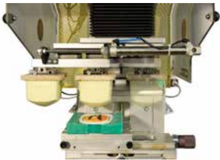
Pad Shuttle 2 to 3 color machines utilize the "RR" / "RRR" pad shuttle function improving multi-color print registration while parts remain stationary.
