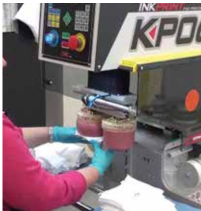
KP06 - 2 Color "RR" printing on fabric. The pad shuttle function, the part remains stationary and the pads move for high quality and precision printing.
