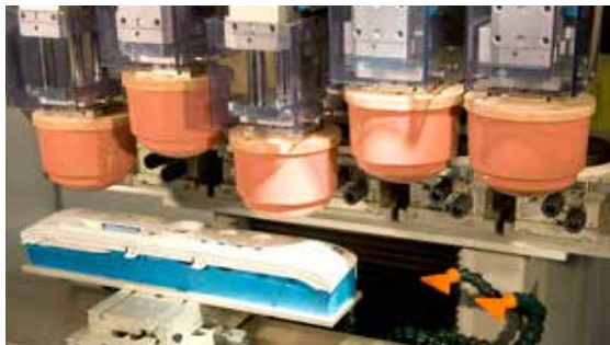
Independent pads - allow larger parts to be printed - with each pad mounted on its own pneumatic cylinder, the pads can operate sequentially or in unison.
