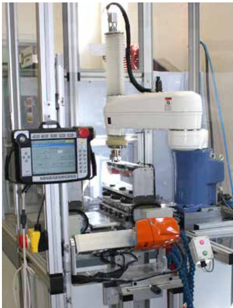
XE-Robot - programmed to select six pads of different shapes and sizes.
