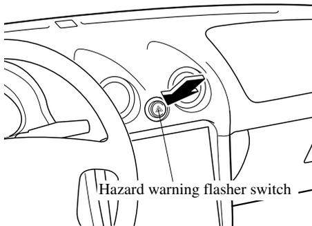
Depress the hazard warning switch and all four turn signals will flash at once.
