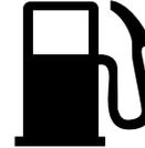
This warning light in the fuel gauge signals that the fuel tank will soon be empty.
