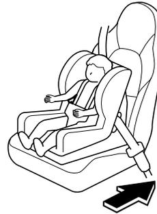
2. Secure the child-restraint system with the lap portion of the lap/shoulder belt. See the instructions on the child-restraint system for belt routing instructions.
