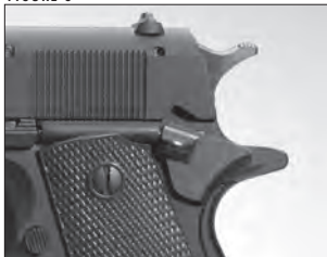
The hammer in the dropped position.
