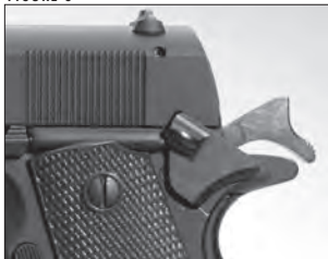
The hammer in the full-cock position.
