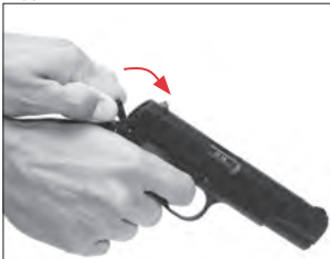
Lowering the hammer to the dropped position.
