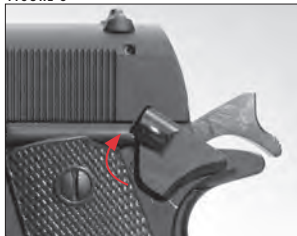
Thumb “safety” shown in the on safe position.
