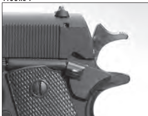
The hammer in the half-cock position.
