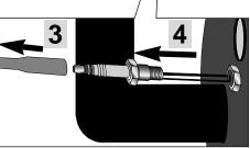
**TIP:** Before removing the spark igniter for inspection, use a felt tip marker to mark the position of the igniter
