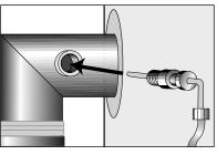
2 Plug the probe's cable into the GasTrac control box. Coil any excess cable and secure with a wire tie.
