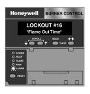
When there is a problem related to the burner or ignition, the burner controller displays a fault code and illuminates an alarm light. To restart the GasTrac after a burner controller alarm:
