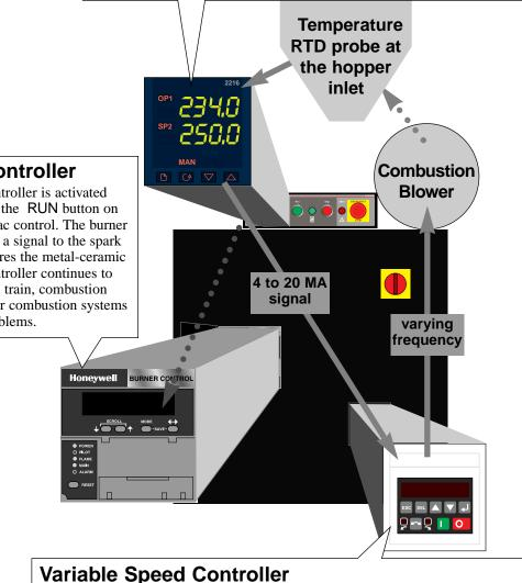
The Variable Speed Controller automatically adjusts the speed of the combustion blower by varying the frequency and voltage of the signal. Increasing the speed increases the air-to-fuel mixture and the heat output of the burner.
