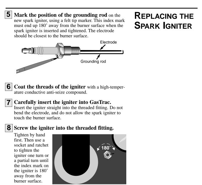
**WARNING:** Do not over tighten the spark igniter. You could damage the porcelain insulator.
