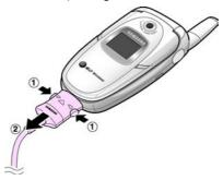
**Note:** You must unplug the adapter before removing the battery from the phone during charging; otherwise, the phone could be damaged.
