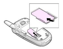
4. Replace the battery so that the tabs on the end align with the slots at the bottom of the phone.
