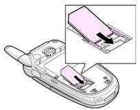
When you need to remove the SIM card, slide it upwards, as shown, and take it out of the socket.
