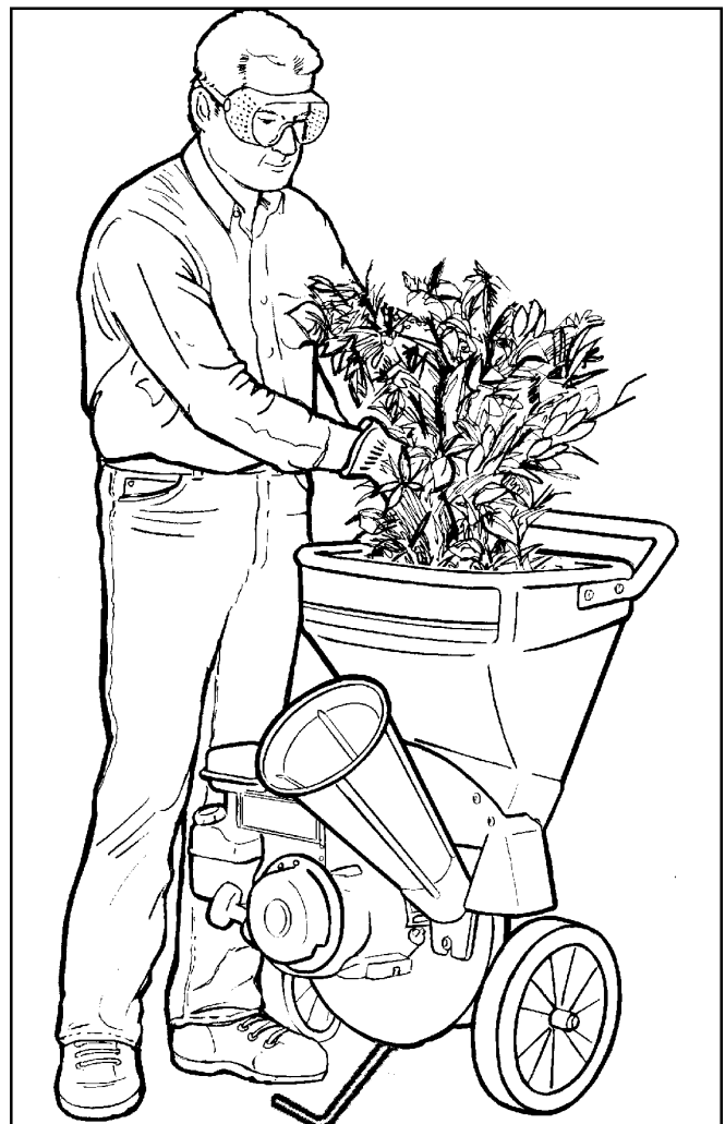
Figure 9. Properly Feeding Longer Materials for Shredding
