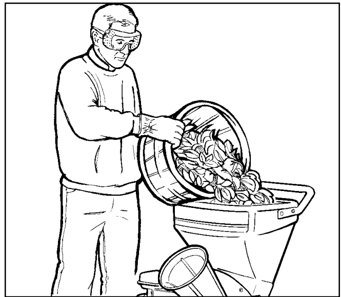
Figure 8. Feeding Materials for Shredding
