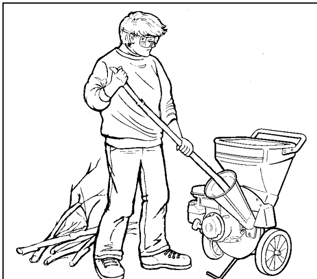
Figure 7. Proper Stance for Chipping
