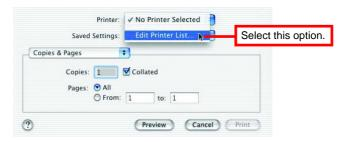
**5.** Click **Add Printer**. Then, select the desired printing protocol (*AppleTalk* or *LPR Printers using IP*).
