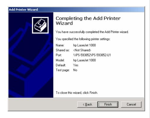
Select the HP Laser Jet 1000 just been added and open the "Property" of it. Click the "Ports" menu and uncheck the "Enable bidirectional support" to make the printing successful.
