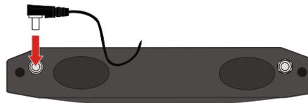
**Figure 1-11 Connect External Power Supply**
