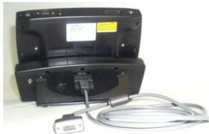
**Figure 1-25 ActiveSync Cable Connected to Serial port on Cradle**
