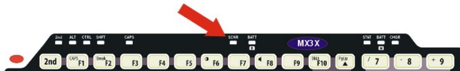
**Figure 1-23 Scanner LED Location**
