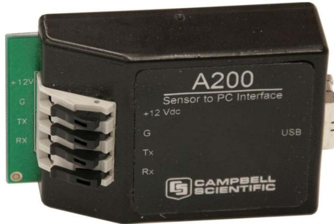
FIGURE 8-1. A200 Sensor-to-PC Interface
