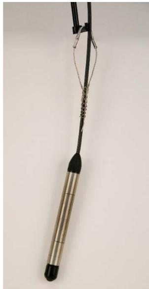
FIGURE 7-1. Transducer suspended with split mesh cable grip
