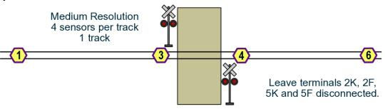
sensor 3, the signal remains on as long as the train is on either sensor 3 or 4. When the train clears both sensor 3 and sensor 4 the signal will turn off. Similar operation occurs when a train travels from right to left.
