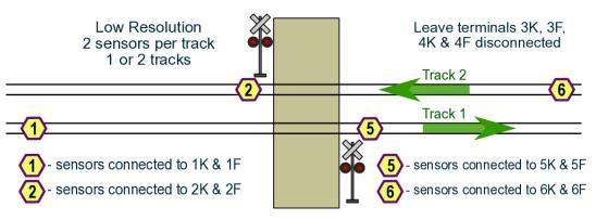
signals will turn off. Similar operation happens if the train on track 1 moves from right to left, encountering sensor 5 first. If trains travel in both directions on a track, place the two sensors equal distances from the crossing. Sensors 2 and 6 on track 2 operate in the same way as the sensors on track 1.
