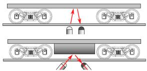
Angle the IR LED and photo receiver so their centerlines intersect at the height of the bottom of your rolling stock.
