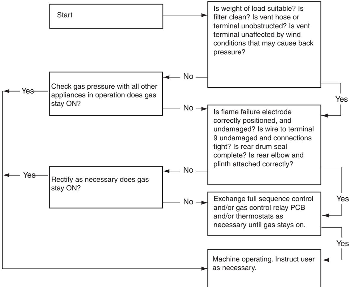
FUNCTIONAL FLOW WIRING DIAGRAM - ECO43A
