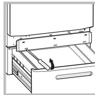
3. Remove the covering panel on the front of the washing machine using a screwdriver (see *figure*);
