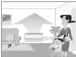
When you go out, push the "HOME LEAVE Operation" button, and the air conditioner will adjust capacity to reach the preset temperature for HOME LEAVE Operation.
