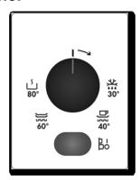
The control panel has a temperature selector and the on/off switch. The control panel is only visible when the drawer is open.
