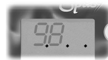
**3 flashing dots are displayed.**
