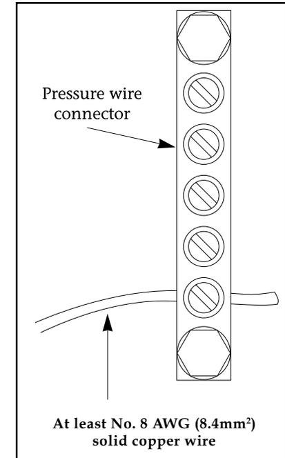
Located on the side of the spa pack box for M Class Equipment Systems and on the heater for S Class Equipment Systems
