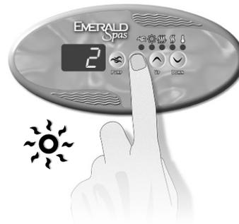
Press and hold Light key for 5 seconds. The display will show a value that represents the filter cycle duration in hours.
