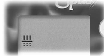
**Pumps have started up for one minute on several occasions and "Filter Cycle" icon is flashing.**
