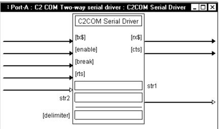
Detail View of an C2COM-3 Device Symbol in SIMPL Windows' Programming Manager
