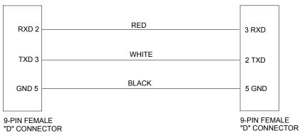
**NOTE:** To support RS-485, tie pin 1 (RXD-) to pin 9 (TXD-) and pin 4 (TXD+) to pin 6 (RXD+) in the cable (refer to the following table).
