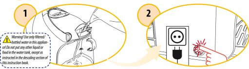
Fill the water tank with filtered/bottled water.
