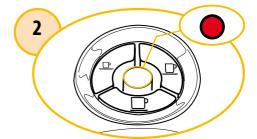
The alarm indicator light will blink and beep three times to confirm deactivation of the "Energy Saving" function. When the function is reactivated, the alarm indicator light will blink and beep two times.
