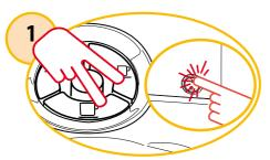
Keep long espresso and brewed coffee/tea buttons pressed down and simultaneously switch machine on.
