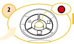
The alarm indicator light will blink and beep. The machine will immediately stop dispensing.
