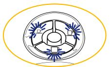
Once the "Energy Saving" function has been programmed, the machine will automatically reduce consumption one hour after the last use. The buttons will slowly blink with a WHITE light.
