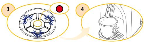
The beverage buttons and alarm indicator light will blink simultaneously.
