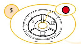
The alarm indicator light will blink and the machine will carry out a drainage cycle. The machine will beep at the end of this cycle.
