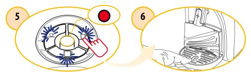
Press the long espresso button. Wait for the machine to complete a rinse cycle. During this cycle, the alarm indicator light will blink. Repeat this step until water is dispensed from the beverage dispensing spout and the alarm indicator light stops blinking. The 3 beverage buttons will blink to confirm end of a rinse cycle.
