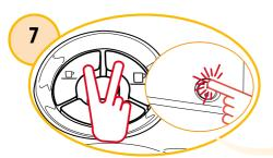
Keep the espresso and long espresso buttons pressed down and simultaneously switch the machine on.
