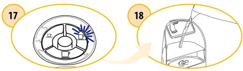
At the end of a rinse cycle, the long espresso button and the descale and alarm indicator lights blink alternately and the machine beeps.
