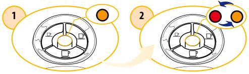
When the descale indicator light blinks and the machine beeps, it is advisable to carry out a descaling cycle.
