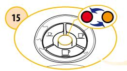
Water will rinse through the machine. During this cycle the descale and alarm indicator lights blink alternately.
