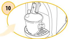
If the container fills up, empty it out. The descale cycle lasts for approximately 40 minutes.
