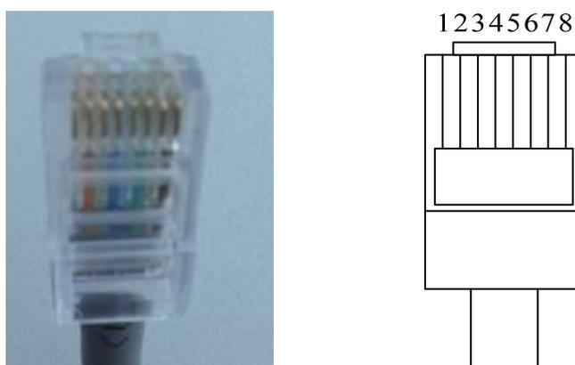
Figure 3-14 Diagram of RS485-1/2 crystal head wiring
