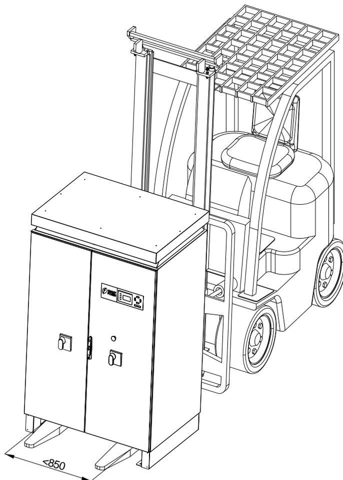
Figure 3-5 Diagram of lifting with a forklift
