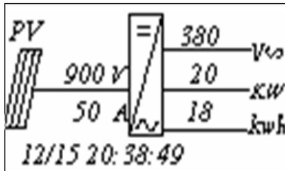
Figure 6-4 Default display interface for normal operation
