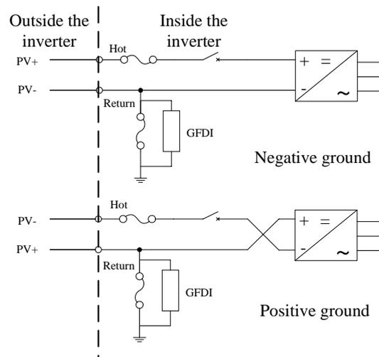
Figure 3-10 Schematic diagram of DC side
