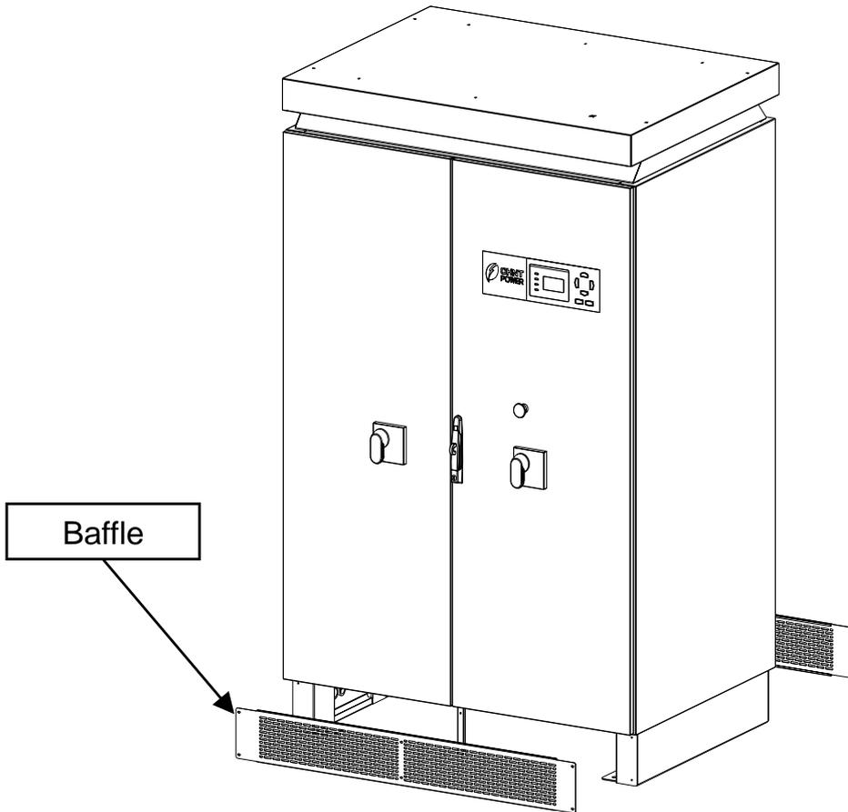
Figure 3-16 Diagram of baffle installation
