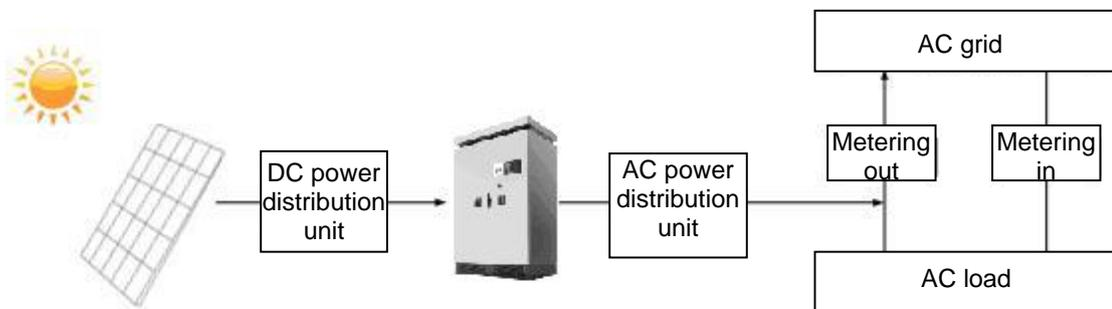
Figure 2-1 Grid connection photovoltaic power generation system
