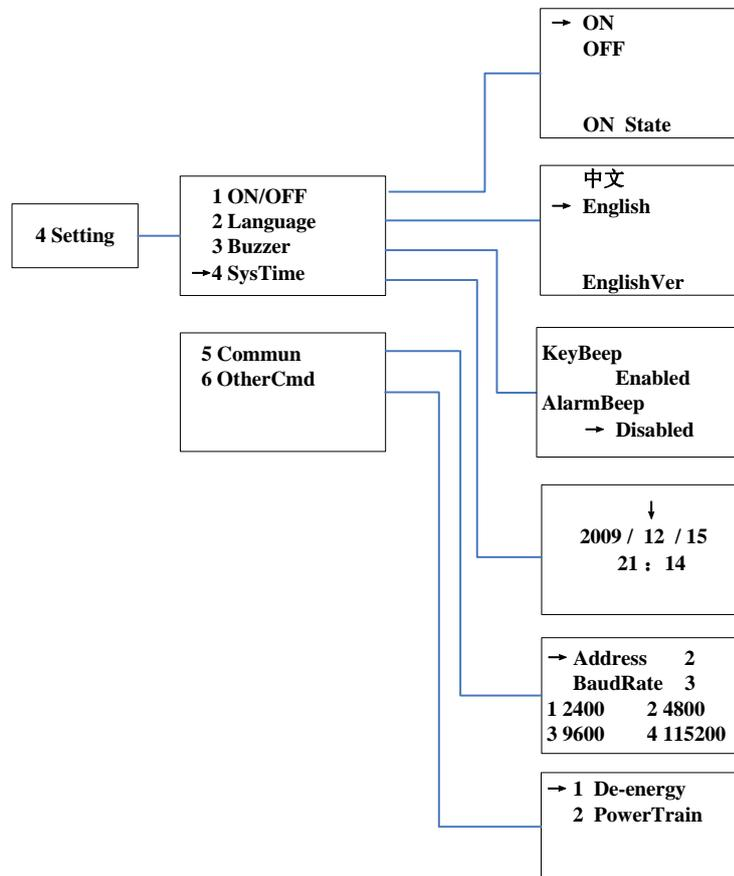
Figure 6-10 System setup menu and submenu
