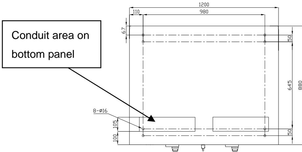
Figure 3-2 Sketch of foundation installation dimensions
