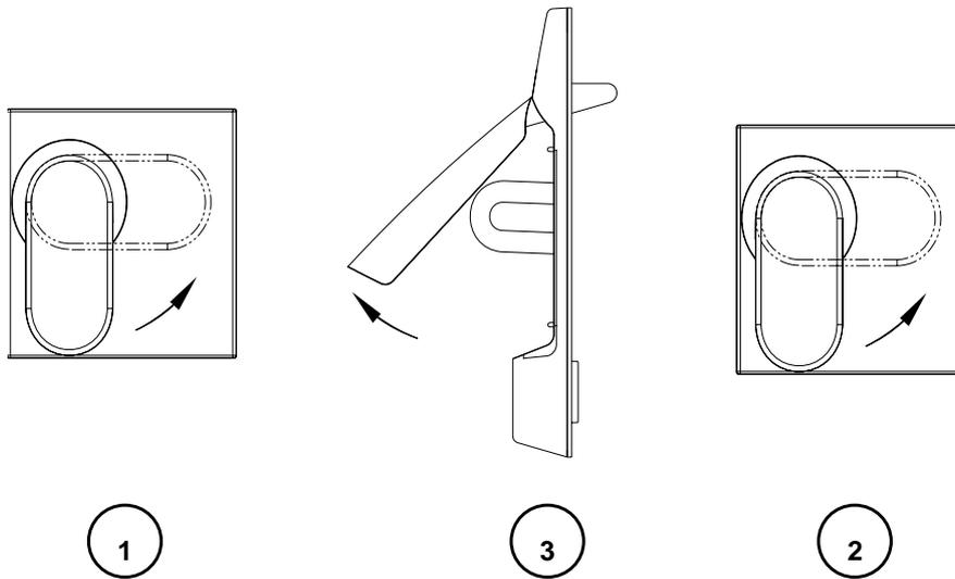
Figure3-6 Diagram of opening front door
