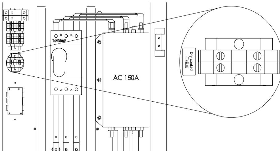
Figure 3-15 Diagram of Dry contact connection
