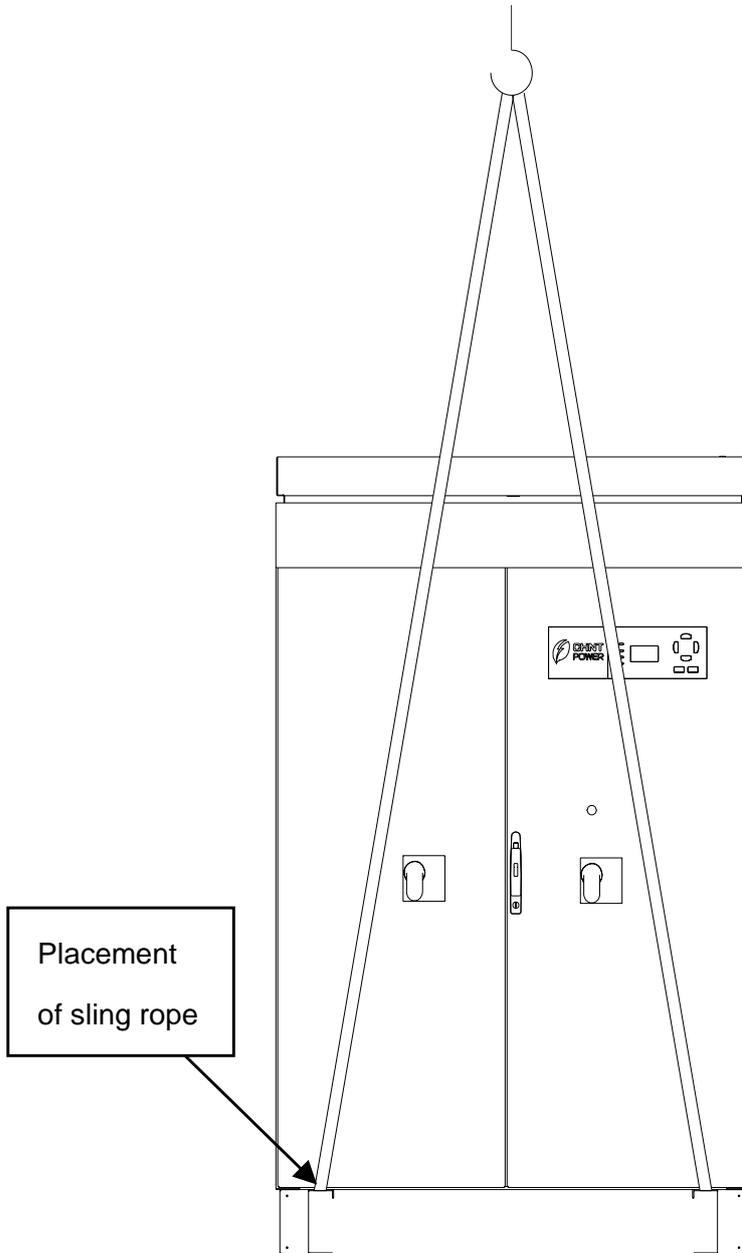
Figure 3-4 Diagram of lifting with a crane
