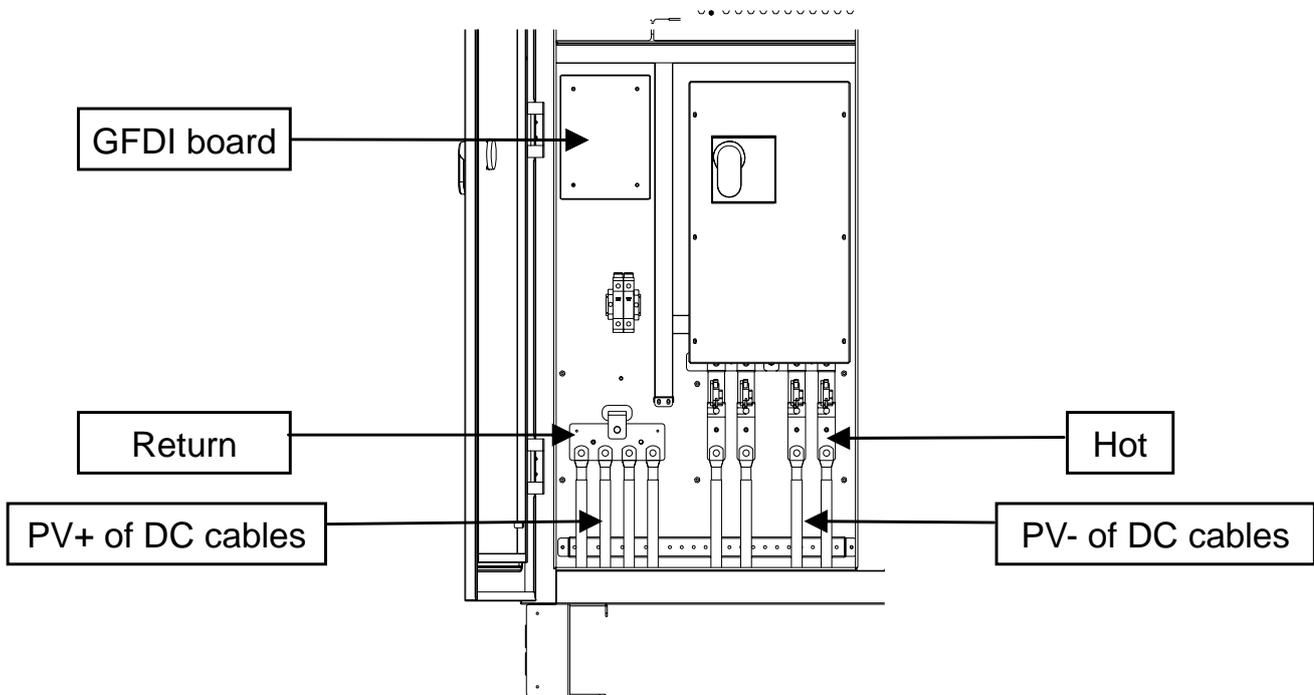
Figure 3-9 DC connection of CPS SC100KT-OPG/US-480
