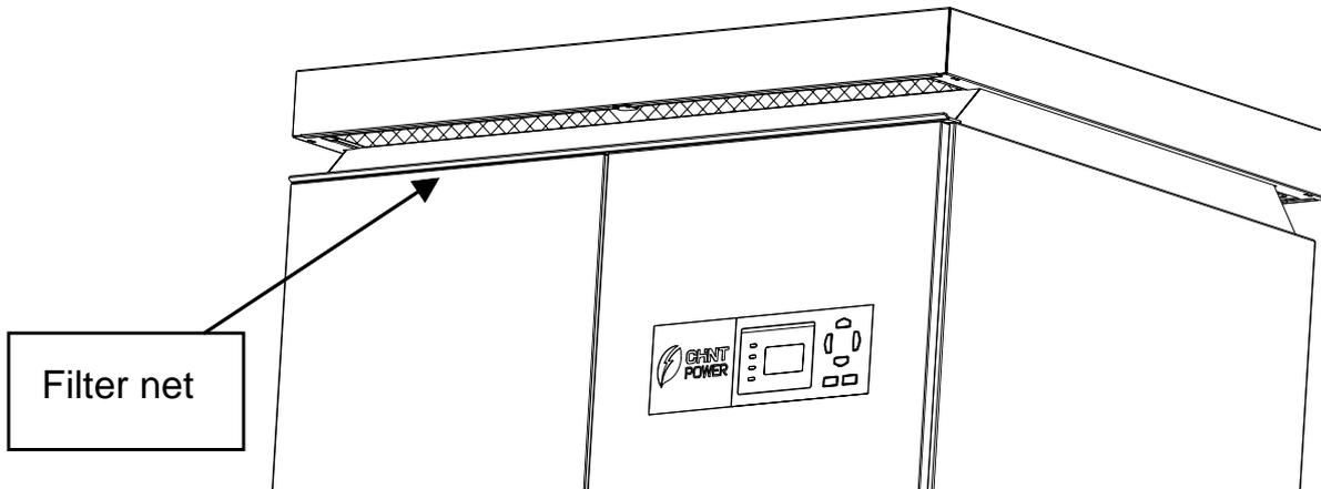
Figure 5-10 Diagram of filter net disassembly (top)
