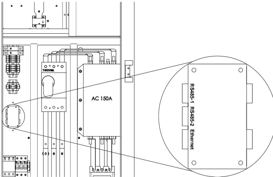
Figure 3-13 Signal cable terminals for communication
