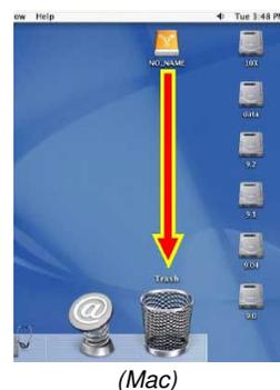
Eject the volume before powering down the unit by dragging the volume's icon to the trash bin, or by selecting the volume then pressing Command-E. Shutting down the unit without first ejecting the volume can result in data loss.
