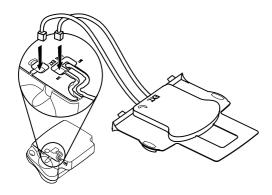
**3** Insert the paper holder with the receiver part of the cordless handset into the openings provided behind the paper feed.
