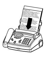
**2** Select the desired resolution with FINE/PHOTO. To make only one copy of the original, briefly press START. The copying process starts immediately.
