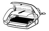
! Do not pull the paper out from the top of the machine because doing so can tear the paper and disrupt the functioning of the fax machine.
