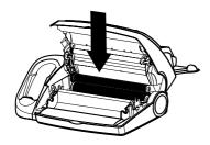
**3** Now take the small roll and lay it in the front ink film compartment. Please make sure that the smaller roller is inserted into the side identations.
