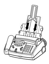
**2** To prevent several sheets being drawn into the machine at once, first fan out the paper to separate the sheets and then straighten the stack on a flat surface before inserting it into the paper feed.
