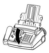
**6** Insert the yellow sheet with the printed side upwards and press START/COPY.
