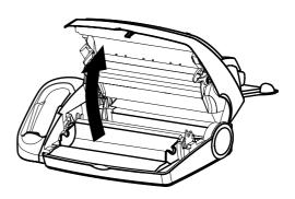
**2** Using a cloth as described above, wipe the printer roller (A). To clean the entire roller turn the roller by hand.
