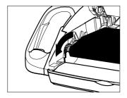
**5** Close the machine by swinging the operation panel forward, until it snaps in.
