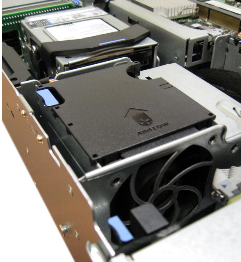
Figure 17. PowerEdge R510-12 Internal View (Redundant PSU with PDB and Additional Fan for PSU)
