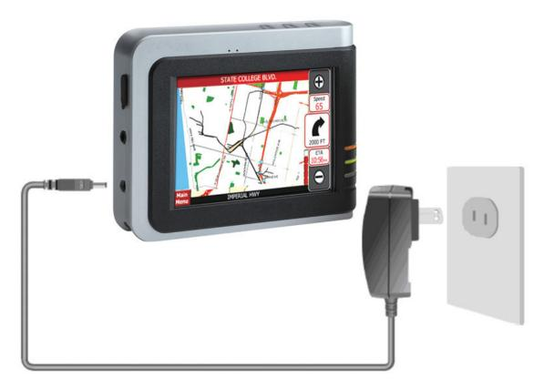
\* The charge indicator glows orange twinkle when charging is in progress. Do not disconnect your device from AC power until the battery is fully charged. This will take a couple of hours.
