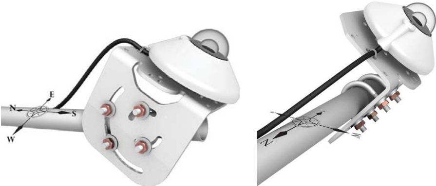
Figure 4-3 Two views of a pyranometer mounted at an angle for the Northern Hemisphere
