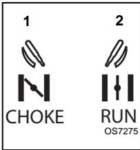
1. Choke Closed position: chokes off air to engine for easier start.
