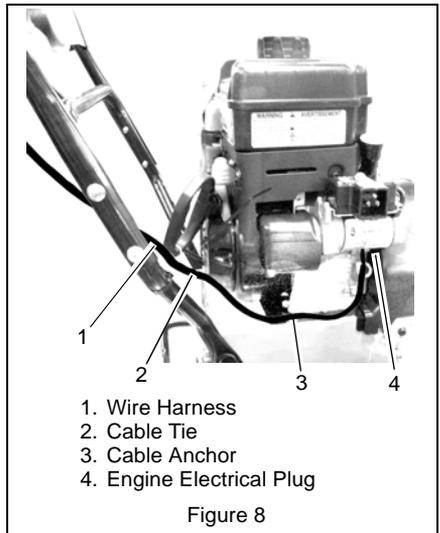
3. Press cable anchor into mounting hole in the frame near the engine electrical plug.
