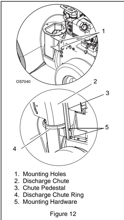
4. Remove the gear cover from top of chute pedestal.
