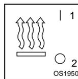
Turn the heated handles switch to the ON (1) position to activate. Turn the switch to the OFF (2) position to deactivate.
