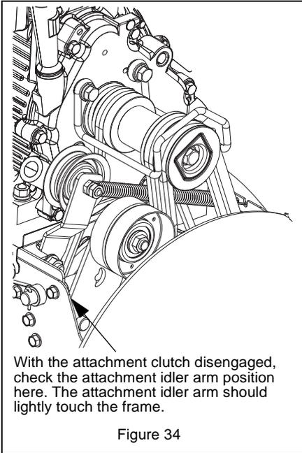
With the attachment clutch disengaged, check the attachment idler arm position here. The attachment idler arm should lightly touch the frame.
