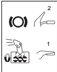
Squeeze Attachment Clutch Lever against handlebar (1) to engage attachment. Release both clutch levers (2) to disengage power and apply brake to attachment.
