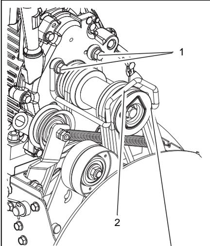
Check belt finger clearance here. With the attachment clutch engaged, there should be less than 1/8" (3 mm) clearance between the belts and the belt finger. The belt finger should not touch the belts.
