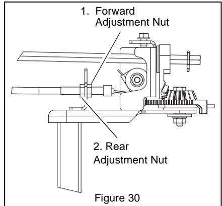
If chute does not rotate freely:
