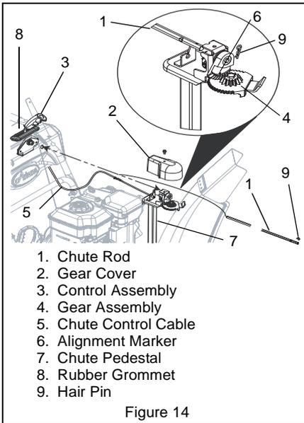
**NOTICE:** To ensure the discharge chute follows its full range of travel, make sure the control lever is centered in the slot and pointing straight up before installing the chute rod.
