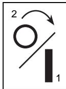
Operate the ignition switch with the removable key. To start the engine, turn the key to Start (1). To stop the engine, turn the key to Off (2).
