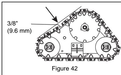
If unit pulls to the left or right when a straight path is desired adjust the track tension. If the unit is pulling to the left, tighten the left track adjuster. If the unit is pulling to the right, tighten the right track adjuster.
