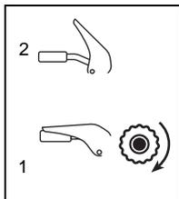
Squeeze the Traction Drive Clutch Lever against the Handlebar (1) to engage wheel drive for propelling unit. Forward speed will vary according to snow depth and moisture content.
