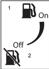
The fuel shut-off valve has two positions:
