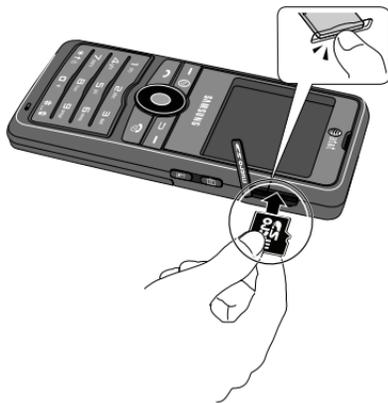
3. To remove the card, a quick press releases the card from the slot.
