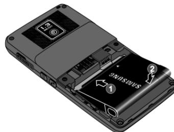
3. With the battery in position on the phone, place the cover back on the handset and slide it in until it clicks.
