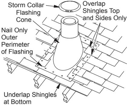
Figure 15 - Flashing Installation
