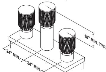
Figure 18 - Multiple Chase Installation
