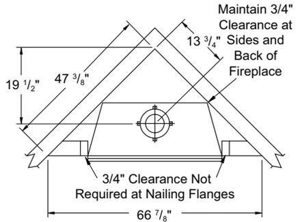
Figure 2 - Corner Installation
