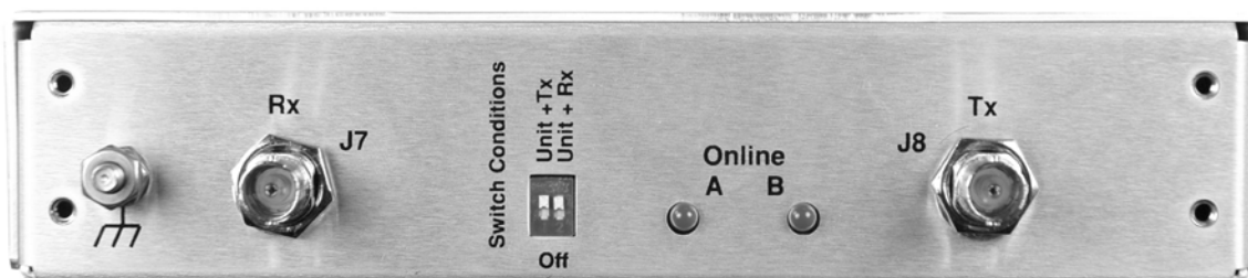
Figure 3-4. CRS-180 – Antenna Side Connectors and Ground Stud
