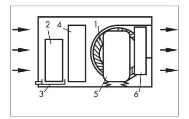
The fan (1) sucks the humid air through the evaporator (2). There the air is cooled and the moisture in the air condenses into water. This water is collected in the tray (3) and drained away through the sump and piping. The compessor (5) pumps the heat, which has been extracted from the air, into the condensor (6). There, this heat is once again released, and absorbed by the dry air. The ready wired control box monitors and controls the operation.
